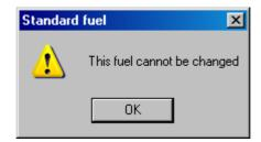
All the other fuels (numbered 10-254) can be defined by the client. The analyser has six programmed standard fuels and the memory holding up to 4 additional fuels defined by the user. The Fuels DataBase window makes it possible for the user to define the new fuels and send their parameters to the analyser when needed.
