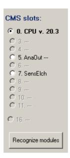
Switching between the analysers (and the available sensors) is carried out by choosing different positions from the list. Marking any of the sensors (or the CPU board) relates all the programme's actions to the chosen element of the analyser.
