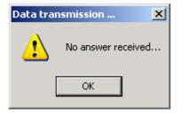
This means the connection process has not been completed successfully, which might have been caused by the inappropriate setting of the serial port in the programme (*Menu > File > Options*) or by a damaged or improper communication cable.
